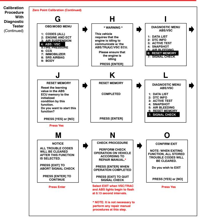
3. Drive the vehicle for at least 5 minutes to confirm Zero Point Calibration is complete.
