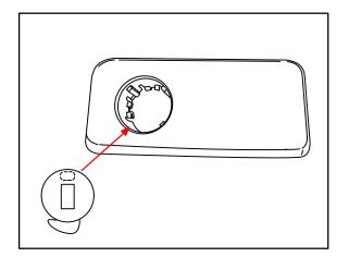
B. With the latch cover facing down, reinstall the spring in the NEW latch assembly.
